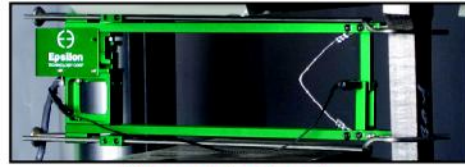
Clip on Extensiyometre Epsilon (Made in USA) MF (Made in Germany) Banner (Made in USA)
